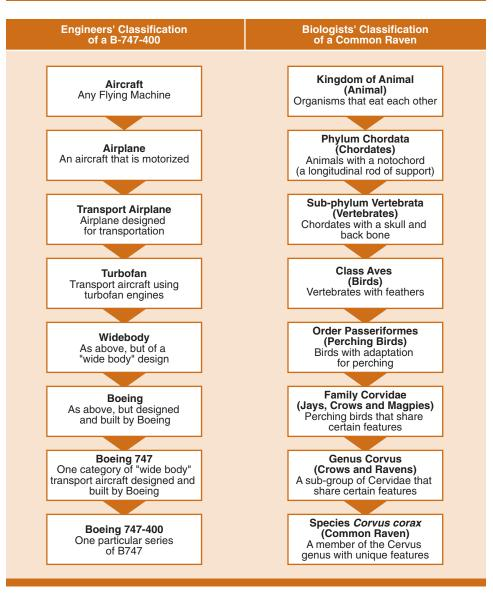
Figure 3.1 Classification of Boeing 747-400 and a Common Raven
