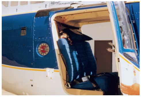
**Plate 6** The impact force of this incident was so severe that after striking the windshield and pilot, the bird damaged the hinges on one rear door.
