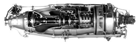
Figure 5.6 Cutaway of a Turboprop Engine
