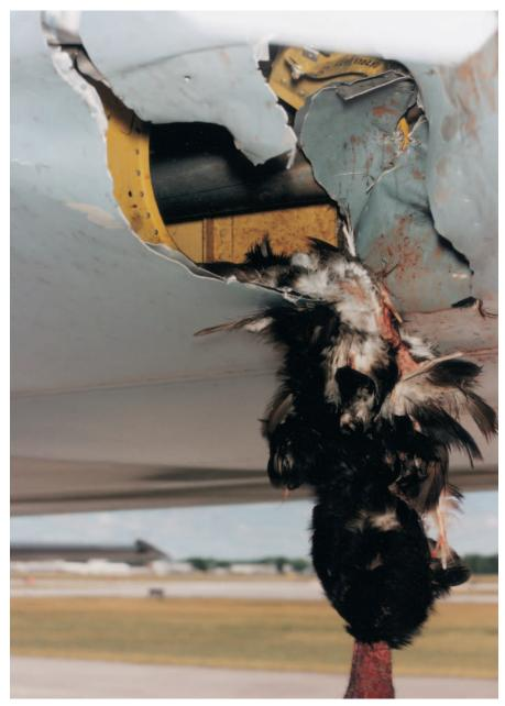
**Plate 12** Severe damage to airframe components and leading edge devices is common in bird strike events. When penetrated to the spar, electrical and hydraulic systems can be affected.
