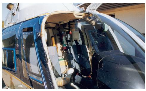
**Plate 5** An impact with a Western Grebe (3 lbs) caused considerable damage to this helicopter. The bird struck the pilot in the face. (See plates 6 and 7)
