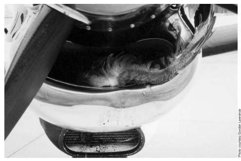
In spite of the protection provided by a propeller, birds can still enter the intakes of turboprop engines, resulting in significant power loss.
