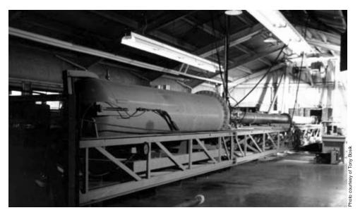
Figure 12.1 Apparatus for testing windshields and airframe components.
