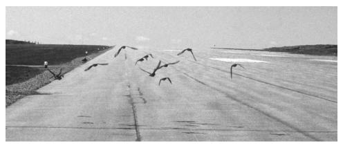
Gulls on runway. The biomass contained in a small flock of gulls is more than any currently operating jet engine is designed to withstand.
