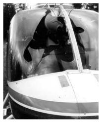
Helicopters operate in environments in which they are highly vulnerable to windshield damage from bird impacts.
