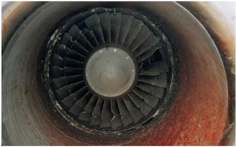
Plate 4 Uncontained engine failure on a Falcon 10 business jet resulting from a bird strike.
