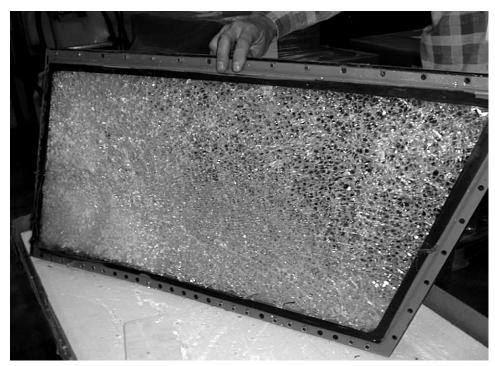
This B737 windshield was damaged as a result of a bird strike at 10,000 ft ASL.
