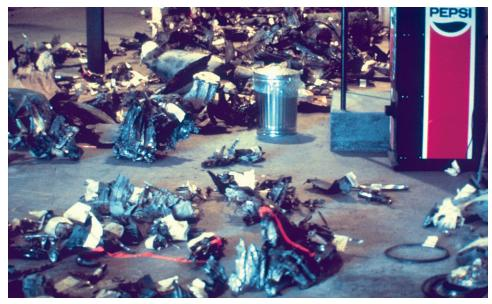
**Plate 8** This is all that remains of a \$200 million USAF B1-B bomber that crashed after striking an American White Pelican in Colorado. The airplane weighed 185,000 lbs, the bird 15 lbs. Three crew members died in the crash.
