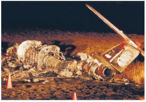
**Plate 13** This RCAF CT-114 Tutor crashed during a training mission over Assiniboia on September 25,1997 after colliding with a single bird. Both crew members ejected safely.
