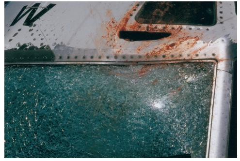
**Plate 11** The windshield on this B737 was severely damaged as a result of a collision with a bird at 10,000 ft. ASL and 250 kts. The captain was injured from debris when the bird penetrated the fuselage above the windshield.
