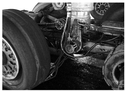
January 2001 in Portland, Oregon. Damage to an MD-11 following rejected takeoff due to bird strike. The aircraft struck a gull at  $V_1$  (167 kts). Other damage included a detached cowl and destruction of one engine.
