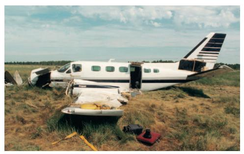
**Plate 3** This accident involving a Cessna 441 Conquest at Fort Frances, Ontario, was the result of a gull being ingested in the intake of the #1 turboprop engine.
