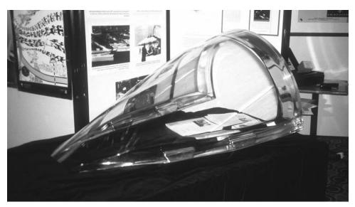
Injection-molded frameless canopies which are very resistant to bird strike damage are being developed by the USAF.
