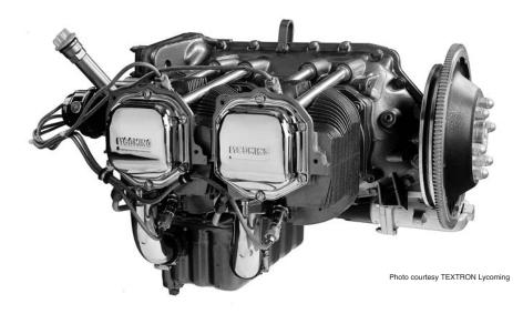
Figure 5.2 Horizontally Opposed Piston Engine
