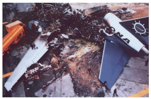
**Plate 9** After striking a gull on takeoff from JKF International Airport on November 12, 1975, the # 3 engine on this ONA DC-10-30 exploded and caused the aircraft to burn out. The 139 passengers, who were all airline employees, safely evacuated the aircraft.
