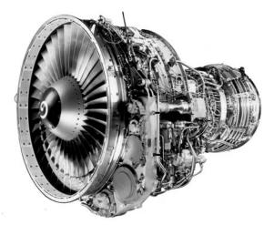
Figure 5.4 CFM56 Turbofan Jet Engine
