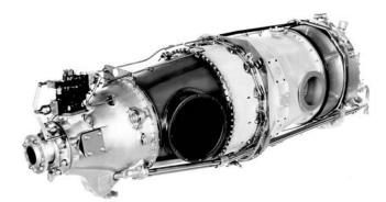
Figure 5.5 PT6 Turboprop Engine
