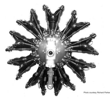
Figure 5.1 Radial Piston Engine
