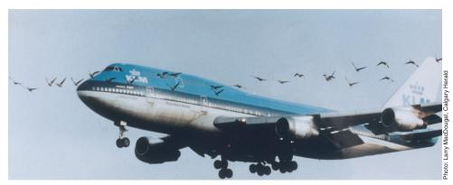
**Plate 10** The # 1 engine on this KLM B-747 suffered an uncontained failure as a result of a collision with Canada Geese while landing at Calgary International Airport. Leading edge devices were also damaged.
