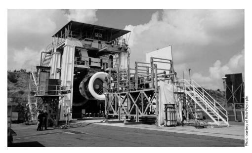
Figure 12.2 Bird impact test facility for jet engines.
