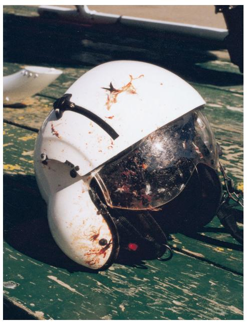
**Plate 7** The helmet and face-shield probably saved the life of the pilot when he was struck in the face by windshield and bird debris.
