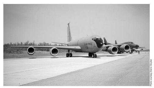
Boeing KC 135. This aircraft is used for air-to-air refuelling.
